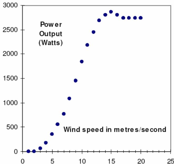
Figure2.4: A typical power curve
