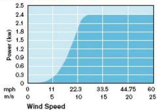
Figure 2.16: Skystream Turbine and power curve
