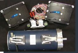
Now here's a steamy bit of kit. High Performance Electric Vehicle Systems (HPEVS) has released a twin rotor 3 phase motor that comes as a kit with two Curtis 1239-8501 controllers, wiring harness, contactor and display. It's actually two AC35 motors built into the same can and on the same shaft driven by two 144v 500A controllers delivering a peak of 257Nm with a peak power of 123Kw and up to 5000rpm. \$10,500 from EVWorks
