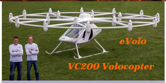
E-volo recently celebrated the maiden launch of its electric two-passenger, 18-rotor VC200 "Volocopter," touting the vehicle's safety and simplicity after an indoor flight inside the dm-arena in Karlsruhe, Germany. Six arms extend from the central part of the rotor ring and split into twelve more arms, with rotors placed at each junction.
