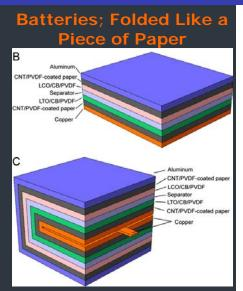
Initial tests showed that by using a simple folding procedure, the batteries with one fold, two folds, and three folds had approximately 1.9, 4.7, and 10.6 times the areal capacity compared to a planar battery. The Coulombic efficiencies for the folded cells were also higher than for the unfolded cell. The Miura folding technique, being highly efficient improves power density to 14X.
