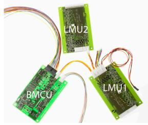
Out of Denmark comes Lithium Balance and their s-BMS. The system is designed around a centralised architecture with a master board (BMCU) communicating over isolated RS485 bus with up to 32 slave boards (LMU). Each slave board can manage 3 - 8 and 2 cells in series temperature sensors. This means a 1000V pack can be safely monitored.
