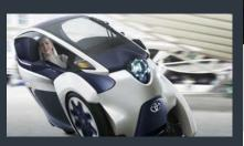
The ultra-compact, three-wheel i-ROAD measures 2,350mm long and 1,445mm high and has a 1,700mm wheelbase. Its most significant dimension, though, is its width: at only 850mm, it is no wider than a conventional motorbike. Not only does this make for easy manoeuvring through congested traffic, it also means four can be parked in a single parking spot. Range is only 50km and maximum speed is just 45kmh but not exciting adequate performance.
