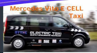
Although announced some little time ago, and has been roaming British streets as a delivery van for almost a year now, the E CELL has been released as a London Taxi. This plug-in electric conversion of the Mercedes Vito van can carry up to six people and has a range of 120 kilometers on a single six hour charge.
