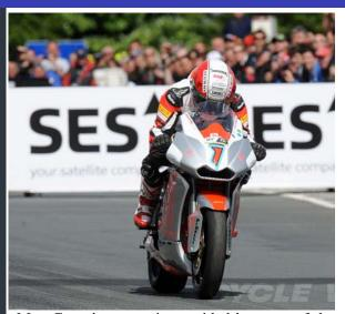
MotoCzysz's power is provided by a set of the latest Dow Kokam lithium-ion nickel-manganese-cobalt cathode cells, which, in comparison with the other four leading cathode chemistries, are claimed to deliver the most "rounded" set of qualities: specific power, specific energy, life, safety, charging time and cost. The motor comes from Remy Electric Motors, their HVH 250 model to be precise, was onboard the two MotoCzysz after a development cycle and redesign by Michael Czysz's.
