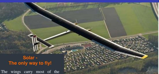
The wings carry most of the 11,628 solar cells on board, but even with more than 185 square meters of photovoltaics, there's not a great deal of energy available to drive the four electric motors.
