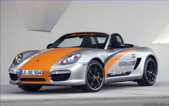
Porsche, having already inspired the EV world with the Hybrid GT3 R and 918 Spyder released the Boxster E all electric at the Michelin challenge in Berlin on May 24<sup>th</sup>. The first Boxster E sports car features two 90kW/270Nm electric motors – one mounted on each axle, the front occupying the space usually filled by the fuel tank – the rear where the transmission usually hangs out!
