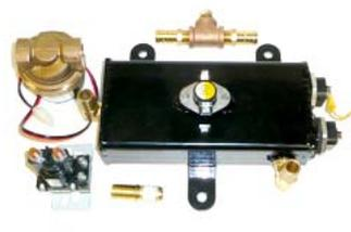
A: Just so happens that EVSource in Utah has a coolant based two stage heater that simply plumbs into the existing ICE cabin heater so you just need to find space under the hood for the package at left, run the heater hose and you're done. Price not cheap \$609
