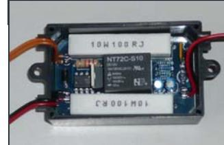
Q: I've got a new speed controller but I'm not sure how to set up a precharge. What options are there?
