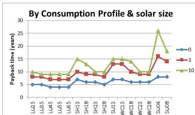
The chart above shows the payback time for those two battery sizes (and no battery) installed in 2017 as part of a 5kW solar system in Sydney, on a flat tariff. In all cases, faster payback is achieved with a smaller battery, and fastest with no battery at all.
