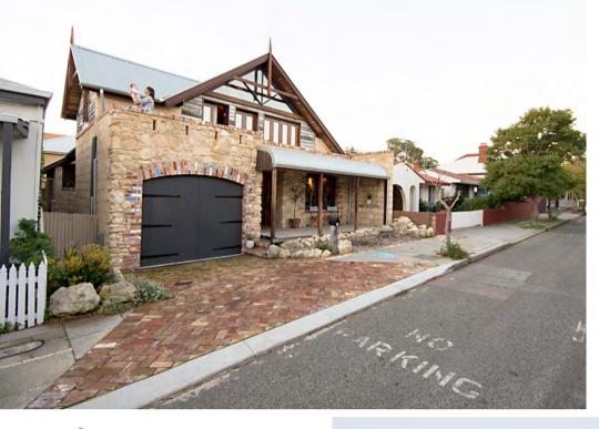
The site features over 80 square metres of broken bricks mostly salvaged from the original house; many were used for the driveway and garage (off-street parking was a council requirement). Instead of the DIY, custom-made thermally broken steel-framed windows used in the rest of the building, timber was used at the front, in order to fit with the heritage precinct.
