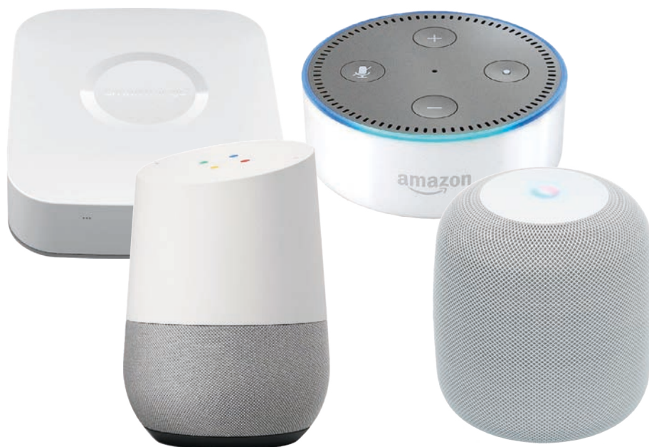
↑ Many smart homes use a hub to tie different devices to the same network. Here are four popular hubs (not to scale), clockwise from top-left: Samsung SmartThings, Amazon Echo Dot, Apple HomePod and Google Home.
