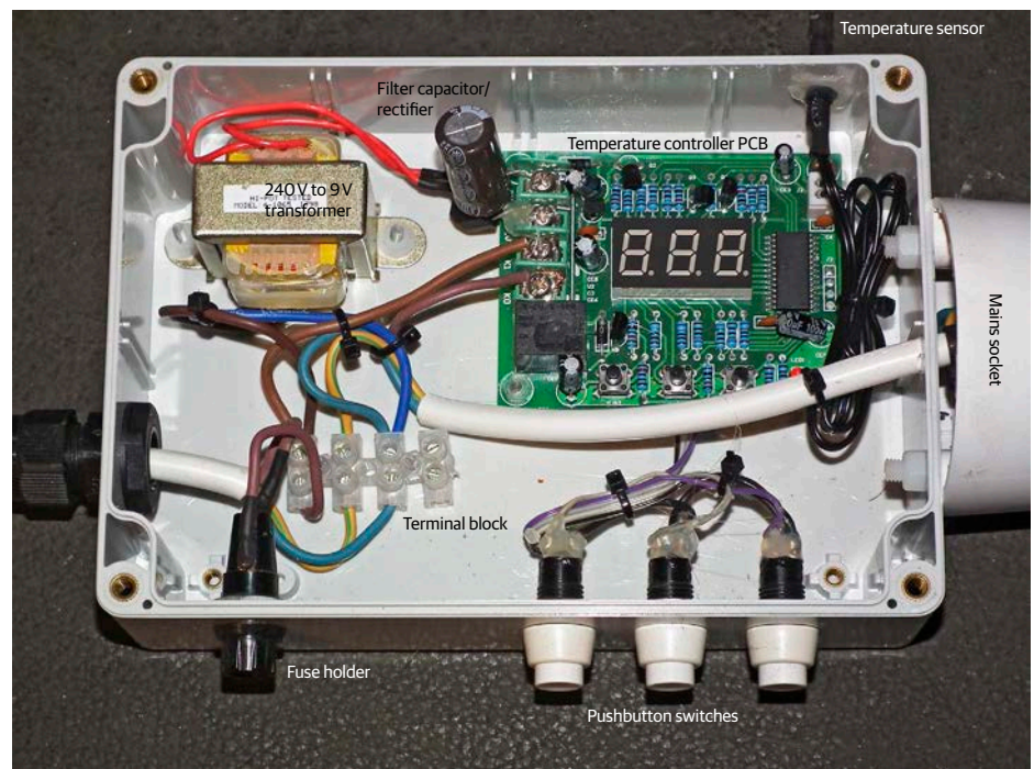
↑ This is the unit I built with cover removed and components labelled. The completed controller is fully insulated for safety. It's not as pretty as a commercially made controller but it is more robust and is easily repairable.
