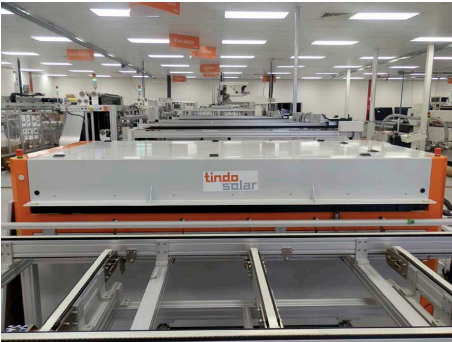
↑ Once the panels are partially assembled they go through the electroluminescence tester to check for defects.
