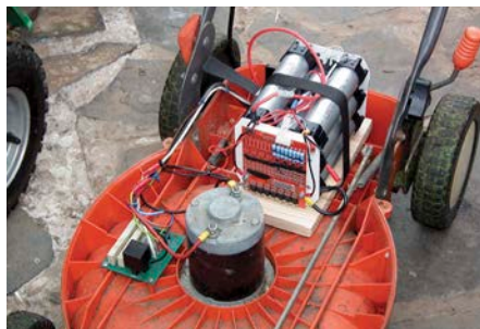
↑ A lithium battery retrofit for a lawnmower. Page 76.
