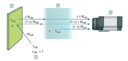
Figure 18.1 A schematic representation of the general thermographic measurement situation.1: Surroundings; 2: Object; 3: Atmosphere; 4: Camera
