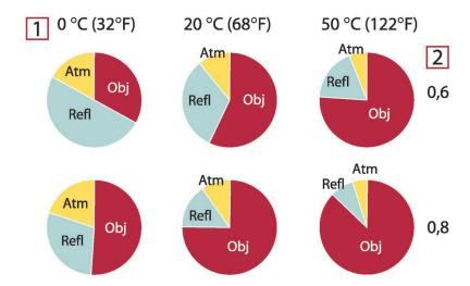
**Figure 18.2** Relative magnitudes of radiation sources under varying measurement conditions (SW camera). 1: Object temperature; 2: Emittance; Obj: Object radiation; Refl: Reflected radiation; Atm: atmosphere radiation. Fixed parameters:  $\tau = 0.88$ ;  $T_{\text{refl}} = 20^{\circ}\text{C}$  (+68°F);  $T_{\text{atm}} = 20^{\circ}\text{C}$  (+68°F).
