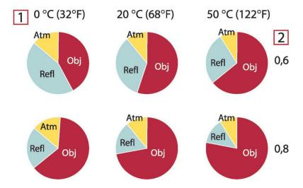
**Figure 18.3** Relative magnitudes of radiation sources under varying measurement conditions (LW camera). 1: Object temperature; 2: Emittance; Obj: Object radiation; Refl: Reflected radiation; Atm: atmosphere radiation. Fixed parameters:  $\tau = 0.88$ ;  $T_{refl} = 20^{\circ}C$  (+68°F);  $T_{atm} = 20^{\circ}C$  (+68°F).
