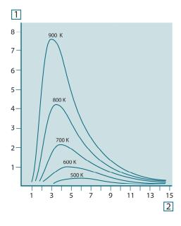
Figure 17.4 Blackbody spectral radiant emittance according to Planck's law, plotted for various absolute temperatures. 1: Spectral radiant emittance (W/cm²  $\times$  10³( $\mu$ m)); 2: Wavelength ( $\mu$ m)
