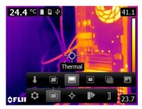
• *Picture-in-picture*: The camera displays a digital camera image with a superimposed infrared image frame.
