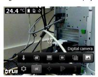
To display a good fusion image (*Thermal MSX*, *Picture-in-picture*, and *Thermal blending* modes), the camera must make adjustments to compensate for the small difference in position between the digital camera lens and the infrared lens. To adjust the image accurately, the camera requires the alignment distance (i.e., the distance to the object).
