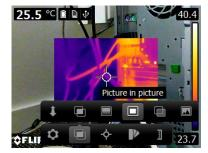
Thermal blending: The camera displays a blended image that uses a mix of infrared pixels and digital photo pixels. The mixing level can be adjusted.
