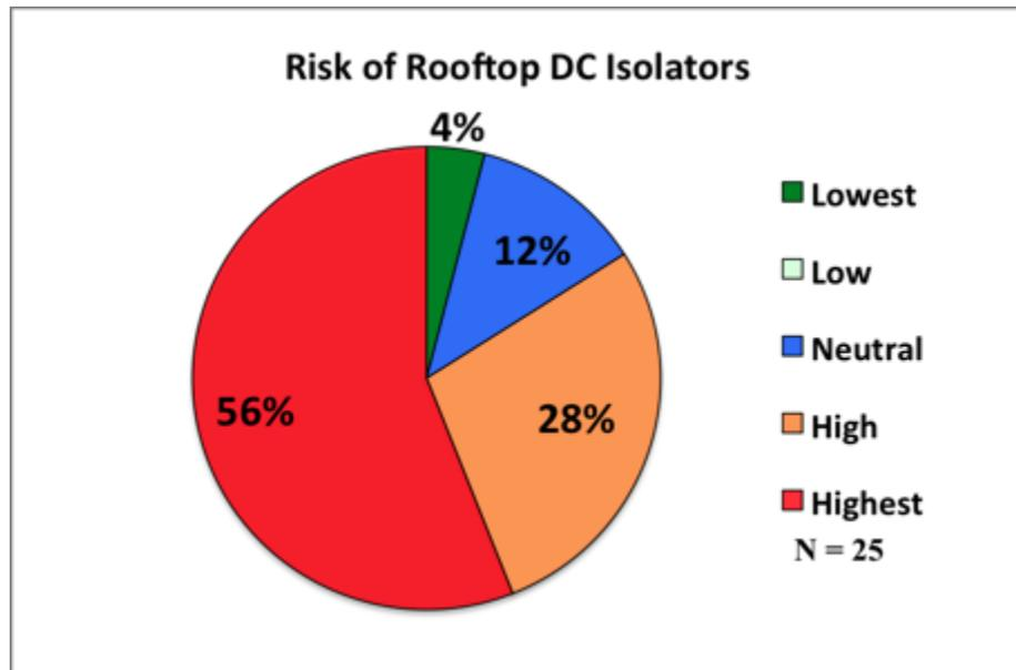
In addition, the majority (84%) of these installers felt that rooftop DC isolators contribute added risk to solar systems. Factors such as harsh weather conditions lead to the breakdown of the system, which can increase the fire risk of the component.
