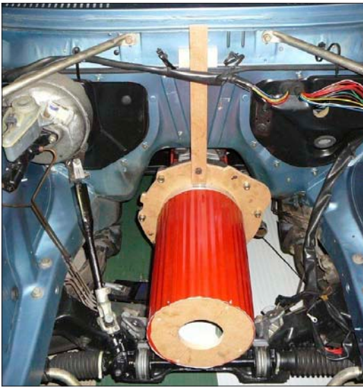
A mockup of the motor was made and attached to the gearbox to ensure the real motor would fit. It's much easier manoeuvring a lightweight motor mockup than the real thing.
