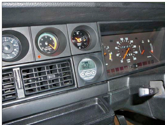
The only visual change to the instruments is the battery monitor, just to the right of the vent.
