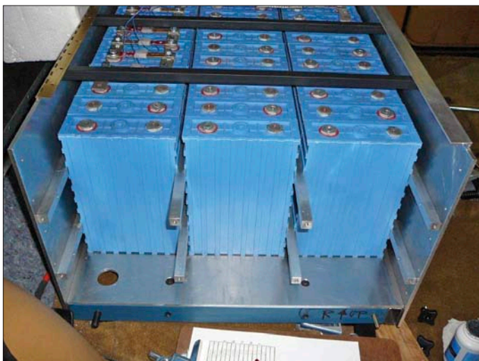
On the left is the battery box being assembled. Note the square section rails between the batteries. At right is the completed and installed battery box, along with the main contactor box.
