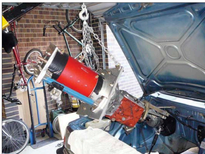
In goes the new electric motor and gearbox. It's a lot smaller than what came out!
